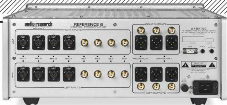
ABOVE: Line-level preamp offers four balanced (on XLR) and four single-ended (on RCA) inputs with pairs of XLR/RCA outputs (plus rec out). RS232 services automation
