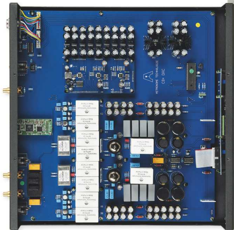
RIGHT: The C8+ is based around a pair of sophisticated 32-bit AK4490 DACs (resampled to 96kHz), features custom passive components and transformer-coupled balanced analogue output stages (solid-state and 6922 tube-based)
