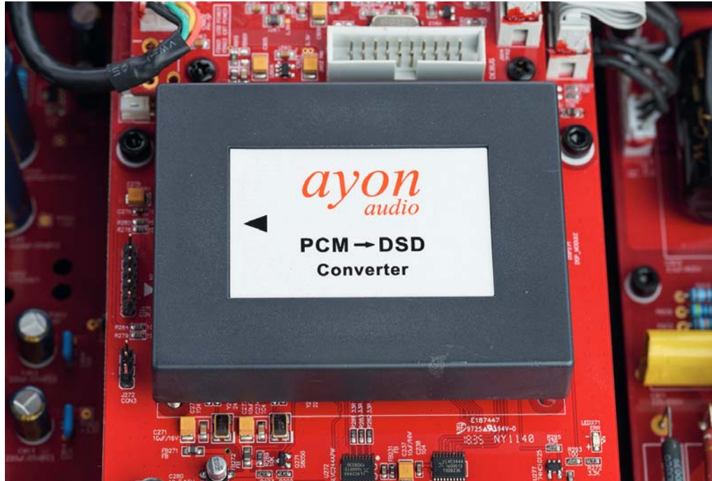
The DSD-module is encapsulated and protected from all too curious glances
