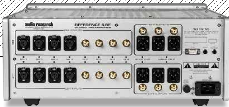
ABOVE: A full eight separate line inputs are offered (four balanced on XLRs and four single-ended on RCAs) with duplicate XLR/RCA record outputs and two sets of XLR/RCA preamp outputs. The latter are variable or fixed in 'processor' mode
