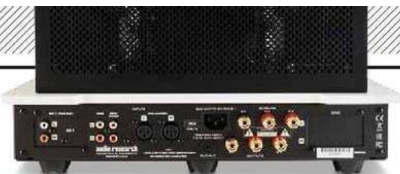
ABOVE: Three single-ended line ins on RCAs (one pass through) and a balanced set on XLRs are joined by 8 and 4ohm speaker taps on gold-plated 4mm binding posts. Note spaces that will accommodate the phono [left] and DAC [right] modules
