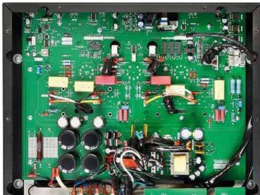
RIGHT: High quality WIMA and Electrocube foil capacitors [red and yellow] feature in the circuit as does logic for the volume and LexieTubes [top]. AC mains and output transformers lie above but note the HT PSU wiring feeding
