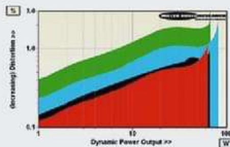
ABOVE: Dynamic power output versus distortion into 8ohm (black trace), 4ohm (red), 2ohm (blue) and 1ohm (green) speaker loads. Maximum current is 8.1A
