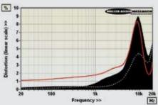
ABOVE: Lateral (L+R, black), vertical (L-R, red), stereo (dotted) tracing and generator distortion (2nd-4th harms) vs. freq. from 20Hz-20kHz (-8dB re. 5cm/sec)
