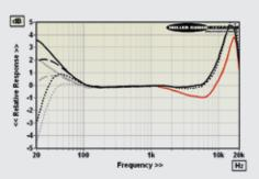
ABOVE: Freq. resp. (-8dB re. 5cm/sec) lateral (L+R, black) vs. vertical (L-R, red) vs. stereo (dashed). Bass only: Output 1/30Hz, solid; 2, dashed; 3, dotted; Output 1/50Hz, grey solid; 2, dotted; 3 dashed)
