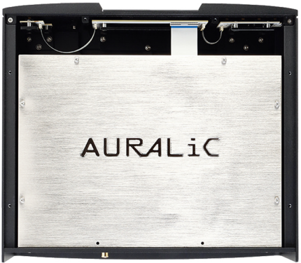
ABOVE: Hidden under the top-plate and screening the digital electronics within is a separate nickel-plated copper enclosure
