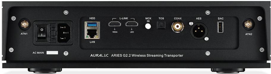
ABOVE: Digital only – the Aries G2.2 offers wired/wireless network control/streaming inputs plus access to more music via internal and external (USB) drives. DSD512 and 384kHz outs are on USB-A, I2S (via HDMI) and DSD64/192kHz on Toslink, coax and AES
