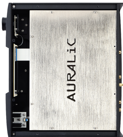
BELOW: Hidden within the alloy chassis, and screening the circuitry within, is a branded nickel-plated copper enclosure
